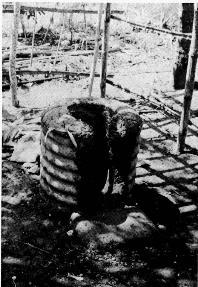
Plate 5. Furnace, moulded within an oil drum, suitable for holding one mould only, built at Kentenkrono.
